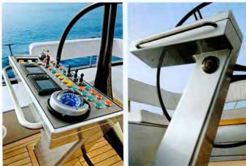
Comfortable manoeuvring: The instruments and controls, including joysticks, on the twin command stations are within arm's reach without awkward twisting.
