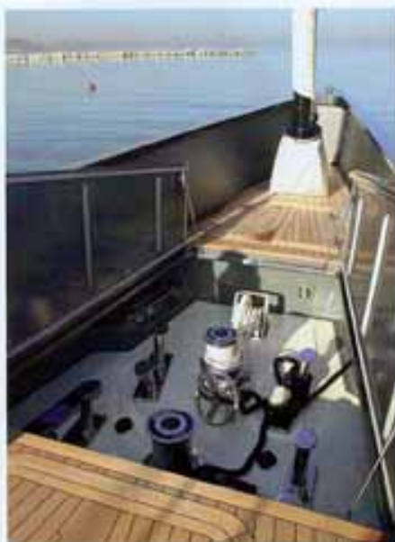
Above: cleats, anchor windlass, warping drum all located below decks. Right: not bad going – 11 knots in 8.4 knots of true wind. And it's early days...
