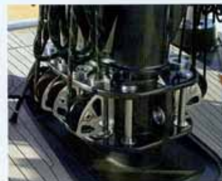
Left: simple controls for mainsheet and blade jib trim on the steering console. Above: Hall Spars have mounted all their turning blocks on a mast collar rather than on the deck
