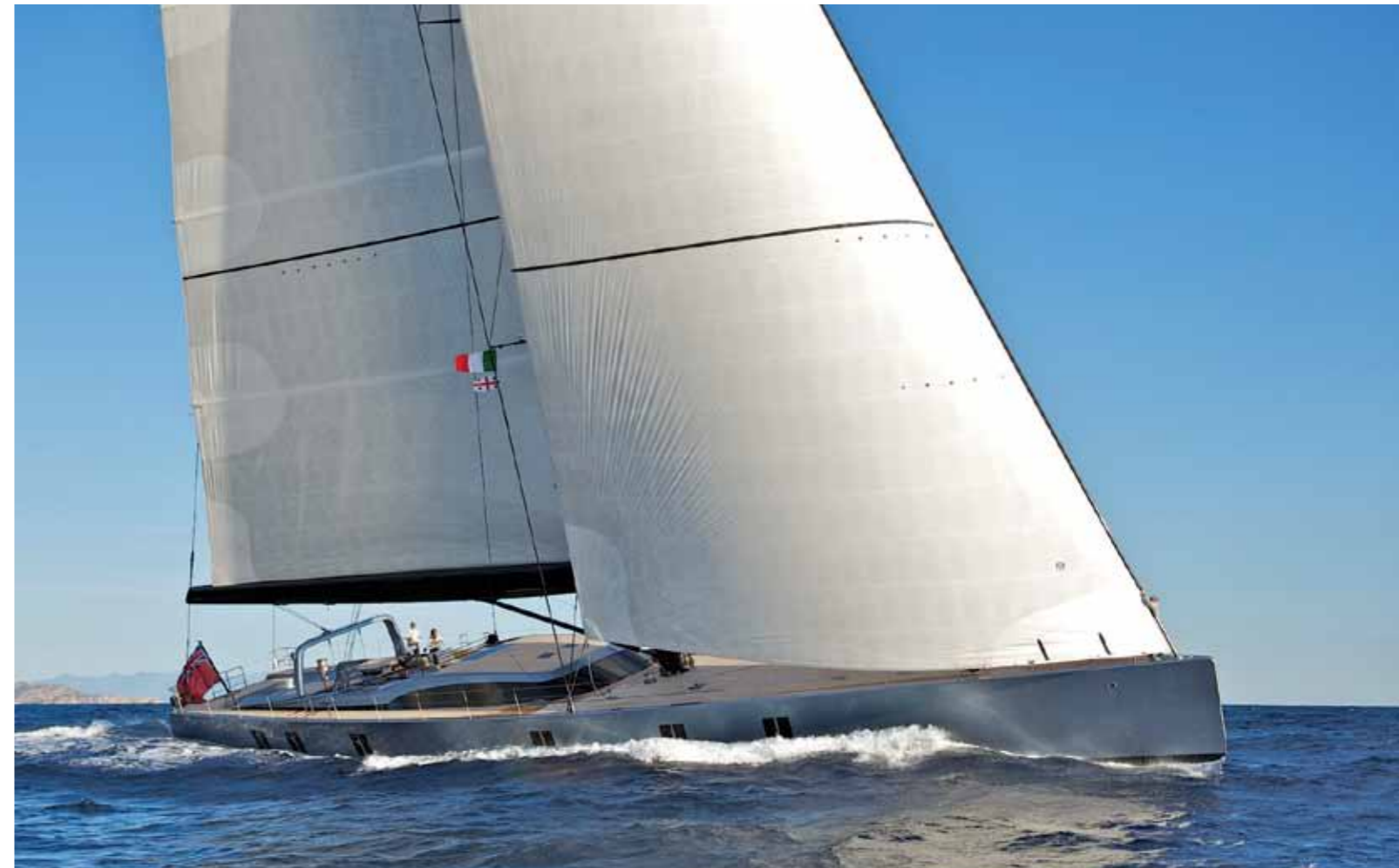
ABOVE: NORTH'S 3DI 107% FURLING GENOA AND FULLY BATTENED IN-BOOM FURLING MAIN. BELOW: TWINNED VERTICAL PORTHOLES EMPHASISE THE HIGH ASPECT RATIO RIG.
