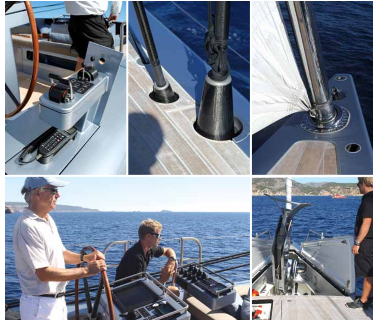
CLOCKWISE (FROM TOP LEFT): POP-UP ENGINE AND THRUSTER CONTROLS. RECESSED EC6+ CARBON SHROUD BASES. RECESSED RECKMANN GENOA HYDRAULIC FURLER WITH ASYMMETRIC FURLER FORWARD. OFFSET CUSTOM GREEN MARINE CARBON HYDRAULIC LAUNCHER FOR 185KG CQR ANCHOR. CLEAR SEPARATION OF STEERING AND SAIL CONTROLS CONSOLES FOR SAFETY.
