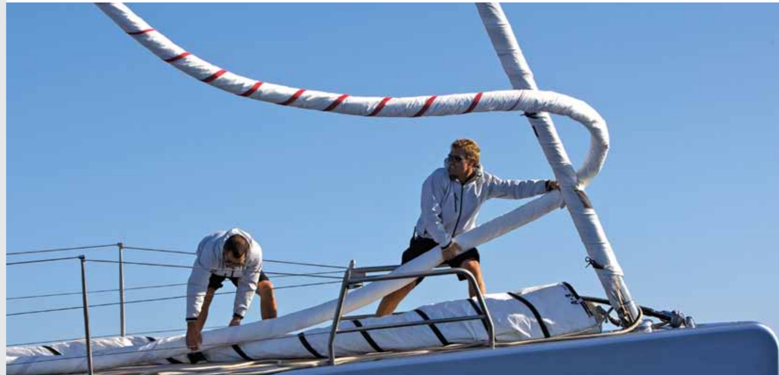
1,150SQM A3 ASYMMETRIC SETS ON A HYDRAULIC CABLE FURLER ON THE BOW.
